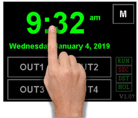
To change any item (other than the am/pm) simply touch and release the button for that item and it is highlighted in green. *The window to the right shows the hours being highlighted.* To change the value touch the plus or minus buttons on the right side and the value in the highlighted button will change accordingly.
