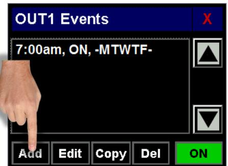
Press the [Add] button and another new event window appears. Touch the [12] hours button and then touch the [+] 8 times to set it to [8]. Then touch the [ON] button to change it to [OFF], and touch the [am] button to change it to [pm]
